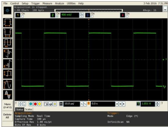
Figure 3. LVCMOS Output Swing ( V_{DD} = 1.8\text{ V} )
