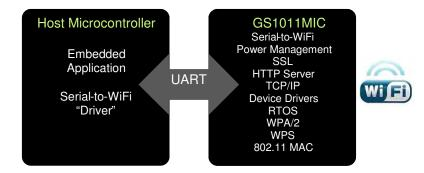
The GS1011 EVK Mrk IIc Evaluation Kit enables GainSpan customers to develop software on their existing microcontrollers to support the "AT" command set, and connect it through the UART interface on the evaluation kit reference board.
