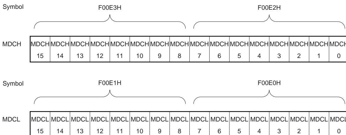
Figure 14-4. Format of Multiplication/Division Data Register C (MDCH, MDCL)
