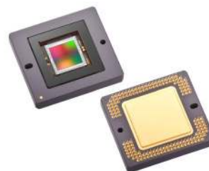
Figure 1. KAE-01093 Interline Transfer EMCCD Image Sensor
