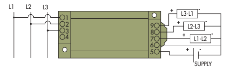
CR4860 3 Element, 3 Wire - 4-20 mA DC Output
