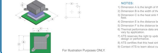
1) Dimension A is the length of the heat sink in the direction of the flow.
