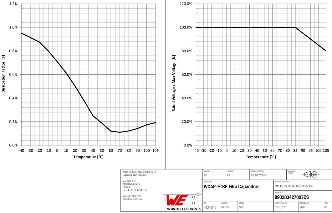
**Rated Voltage vs. Temperature:**
