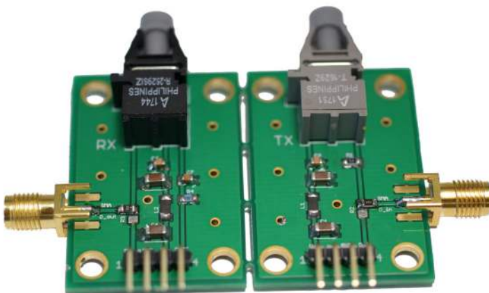
Figure 6: Modified Interfaces with SMA Connectors for Tx Input and Rx Output Signals
