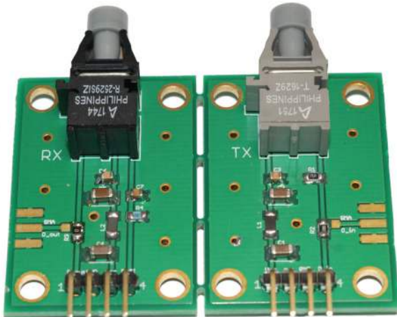
Figure 6: Modified Interfaces with SMA Connectors for Tx Input and Rx Output Signals
