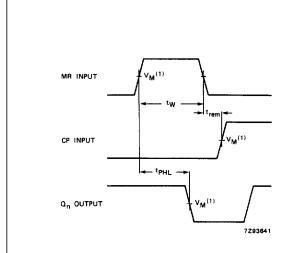
(1) HC :  $V_M$  = 50%;  $V_I$  = GND to  $V_{CC}$ . HCT:  $V_M$  = 1.3 V;  $V_I$  = GND to 3 V.
