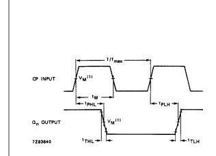
(1) HC :  $V_M$  = 50%;  $V_I$  = GND to  $V_{CC}$ . HCT:  $V_M$  = 1.3 V;  $V_I$  = GND to 3 V.
