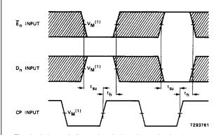
The shaded areas indicate when the input is permitted to change for predictable output performance.
