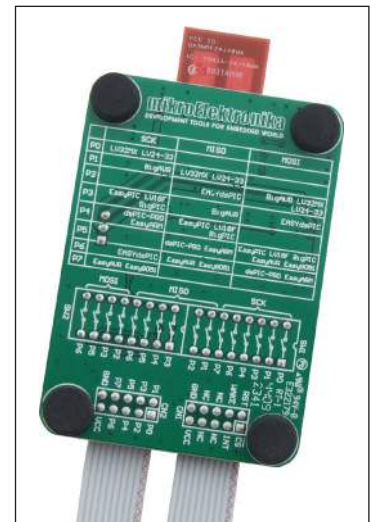
Figure 2: Back of the Easy Bee3 board
