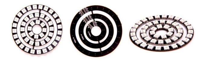
An upgraded version of WS2812. This is the 48 RGB Led ring in natural white. The RGB LED Ring are 5050-sized LEDs with an embedded microcontroller inside the LED.
