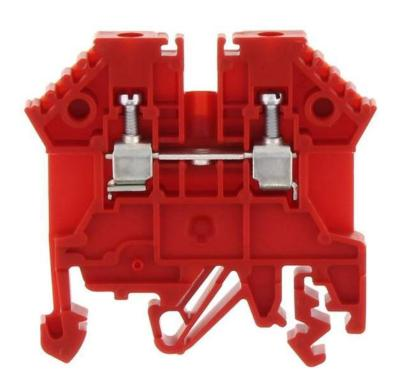
Feed-through terminal, Screw connection, Mounting type:Mounting rail TS 35/7.5 and TS 32, Rated cross-section: 2.5 mm², Width: 5 mm, Colour: Red
