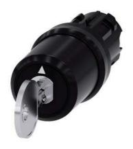
key-operated switch Siemens, 22 mm, round, plastic, lock number SSG10, with 2 keys, 3 switch positions I>O<II, momentary contact on the left, latching on the right, actuating angle  $2x45^{\circ}$ , 10:30h/12h/13:30h, key removal O+II, with laser labeling, upper case and lower case, always upper case at the beginning of the word
