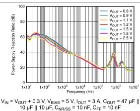
Figure 6-5. PSRR vs Frequency and V<sub>OUT</sub> With Bias
