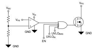
Figure 7-6. Simplified PG Circuit
