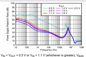
= 5 V,  $I_{OUT}$  = 3 A,  $C_{OUT}$  = 47  $\mu F$  || 10  $\mu F$  || 10  $\mu F$ ,  $C_{NR/SS} = 10 \text{ nF}, C_{FF} = 10 \text{ nF}$
