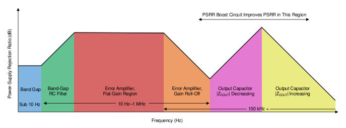
Figure 8-6. Power-Supply Rejection Ratio Diagram
