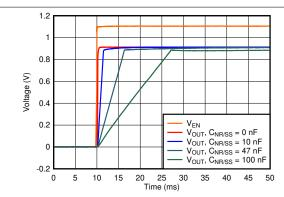
$V_{IN}$  = 1.2 V,  $V_{OUT}$  = 0.9 V,  $V_{BIAS}$  = 5 V,  $I_{OUT}$  = 3 A,  $C_{OUT}$  = 47  $\mu$ F || 10  $\mu$ F || 10  $\mu$ F,  $C_{FF}$  = 10 nF
