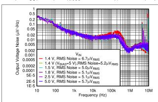
$V_{OUT}$  = 0.7 V,  $I_{OUT}$  = 3 A,  $C_{OUT}$  = 47  $\mu$ F || 10  $\mu$ F || 10  $\mu$ F,  $C_{NR/SS}$  = 10 nF,  $C_{FF}$  = 10 nF, RMS noise BW = 10 Hz to 100 kHz
