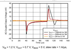
Figure 6-65. Load Transient vs Time and DC Load
