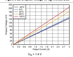
Figure 6-22. Dropout Voltage vs I<sub>OUT</sub> Without Bias
