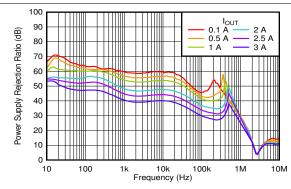
$V_{IN} = 5.5 \text{ V}, V_{OUT} = 5 \text{ V}, I_{OUT} = 3 \text{ A}, C_{OUT} = 47 \mu\text{F} \parallel 10 \mu\text{F} \parallel 10 \mu\text{F}, C_{NR/SS} = 10 \text{ nF}, C_{FF} = 10 \text{ nF}$
