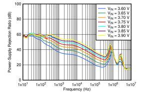
$I_{OUT}$  = 3 A,  $C_{OUT}$  = 47  $\mu$ F || 10  $\mu$ F || 10  $\mu$ F,  $C_{NR/SS}$  = 10 nF,  $C_{FF}$  = 10 nF
