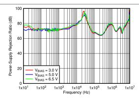
$V_{IN}$  =  $V_{OUT}$  + 0.3 V,  $V_{OUT}$  = 1 V,  $I_{OUT}$  = 3 A,  $C_{OUT}$  = 47  $\mu F$  || 10  $\mu F$  || 10  $\mu F$  ,  $C_{NR/SS}$  = 10 nF,  $C_{FF}$  = 10 nF
