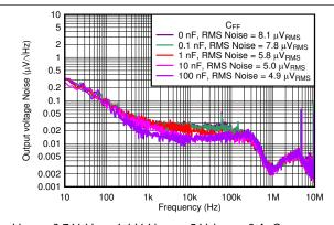
$V_{OUT}$  = 0.7 V,  $V_{IN}$  = 1.1 V,  $V_{BIAS}$  = 5 V,  $I_{OUT}$  = 3 A,  $C_{OUT}$  = 47  $\mu F$  || 10  $\mu F$  || 10  $\mu F$ ,  $C_{NR/SS}$  = 10 nF, RMS noise BW = 10 Hz to 100 kHz
