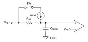
Figure 7-4. Simplified Soft-Start Circuit
