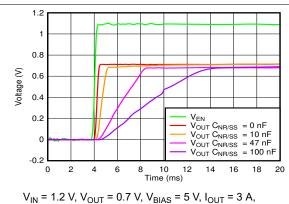
$C_{OUT} = 47 \mu F || 10 \mu F || 10 \mu F, C_{FF} = 10 nF$
