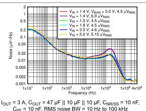
Figure 6-11. Output Noise vs Frequency and V<sub>IN</sub>
