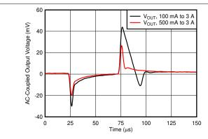
$V_{IN}$  = 1.2 V,  $V_{BIAS}$  = 5 V,  $C_{OUT}$  = 47  $\mu F$  || 10  $\mu F$  || 10  $\mu F$  ,  $V_{OUT}$  = 0.9 V,  $C_{NR/SS}$  =  $C_{FF}$  = 10 nF, slew rate = 1 A/ $\mu s$
