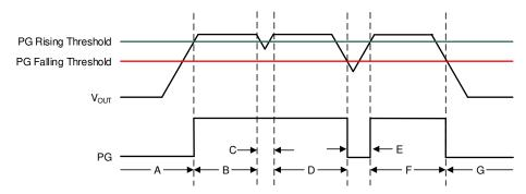
Figure 8-5. Typical PG Operation
