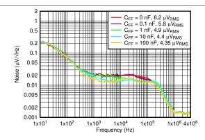
$V_{IN}$  =  $V_{OUT}$  + 0.3 V,  $V_{BIAS}$  = 5 V,  $I_{OUT}$  = 3 A,  $C_{OUT}$  = 47  $\mu F$  || 10  $\mu F$  || 10  $\mu F$  ,  $C_{NR/SS}$  = 10 nF, RMS noise BW = 10 Hz to 100 kHz
