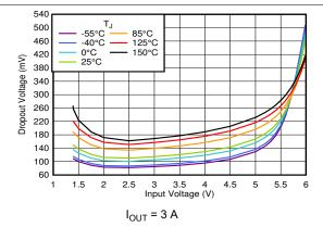
Figure 6-66. Dropout Voltage vs V<sub>IN</sub> Without Bias
