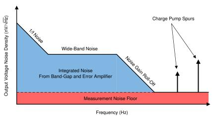
Figure 8-7. Output Voltage Noise Diagram
