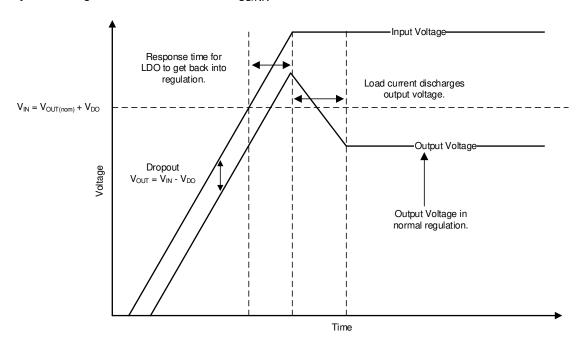
Figure 8-12. Start-Up Into Dropout
