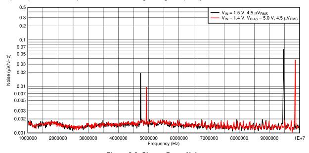
Figure 8-8. Charge Pump Noise
