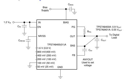
Figure 8-21. TPS7A84A Typical Application
