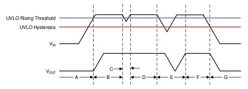
Figure 8-4. Typical UVLO Operation
