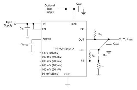
Figure 8-1. Adjustable Operation
