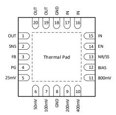
Figure 5-2. RGR Package (TPS7A8401A), 20-Pin VQFN, Top View
