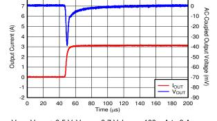
$V_{IN}$  =  $V_{OUT}$  + 0.5 V,  $V_{OUT}$  = 0.7 V,  $I_{OUT}$  = 100 mA to 3 A,  $C_{OUT}$  = 47  $\mu F$  || 10  $\mu F$  || 10  $\mu F$ ,  $C_{NR/SS}$  =  $C_{FF}$  = 10 nF, slew rate = 1 A/ $\mu s$
