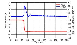
$V_{IN} = V_{OUT} + 0.5 \text{ V}, V_{OUT} = 0.7 \text{ V}, I_{OUT} = 3 \text{ A to } 100 \text{ mA},$   $C_{OUT} = 47 \mu\text{F} \parallel 10 \mu\text{F} \parallel 10 \mu\text{F}, C_{NR/SS} = C_{FF} = 10 \text{ nF, slew rate}$ = 1 A/us
