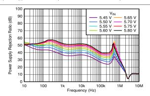
$V_{OUT}$  = 5 V,  $I_{OUT}$  = 3 A,  $C_{OUT}$  = 47  $\mu$ F || 10  $\mu$ F || 10  $\mu$ F,  $C_{NR/SS}$  = 10 nF,  $C_{FF}$  = 10 nF
