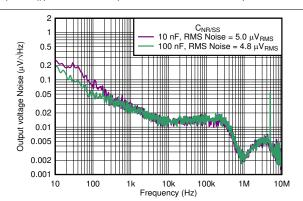
$V_{OUT}$  = 0.7 V,  $V_{IN}$  = 1.1 V,  $V_{BIAS}$  = 5 V,  $I_{OUT}$  = 3 A,  $C_{OUT}$  = 47  $\mu F$  || 10  $\mu F$  || 10  $\mu F$ ,  $C_{FF}$  = 10 nF, RMS noise BW = 10 Hz to 100 kHz
