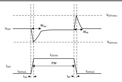
Figure 8-10. Simplified Load Transient Waveform
