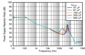
$V_{IN}$  = 1.4 V,  $V_{BIAS}$  = 5 V,  $V_{OUT}$  = 1 V,  $I_{OUT}$  = 3 A,  $C_{NR/SS}$  = 10 nF,  $C_{FF}$  = 10 nF
