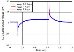
$V_{OUT}$  = 5 V,  $I_{OUT, DC}$  = 100 mA,  $I_{OUT}$  = 100 mA to 3 A,  $C_{OUT}$  = 47  $\mu$ F  $\parallel$  10  $\mu$ F  $\parallel$  10  $\mu$ F,  $C_{NR/SS}$  =  $C_{FF}$  = 10 nF
