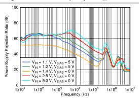
$I_{OUT}$  = 1 A,  $C_{OUT}$  = 47  $\mu$ F || 10  $\mu$ F || 10  $\mu$ F,  $C_{NR/SS}$  = 10 nF,  $C_{FF}$  = 10 nF
