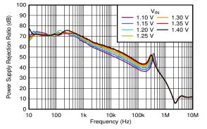
$I_{OUT} = 3 \text{ A}, V_{BIAS} = 5 \text{ V}, C_{OUT} = 47 \mu\text{F} \parallel 10 \mu\text{F} \parallel 10 \mu\text{F},$  $C_{NR/SS} = 10 \text{ nF}, C_{FF} = 10 \text{ nF}$
