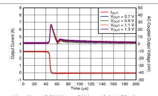
$$\begin{split} V_{\text{IN}} = V_{\text{OUT}} + 0.5 \text{ V, } V_{\text{BIAS}} = 5 \text{ V, } I_{\text{OUT}} = 3 \text{ A to } 100 \text{ mA,} \\ \text{slew rate} = 1 \text{ A/µs, } C_{\text{NR/SS}} = C_{\text{FF}} = 10 \text{ nF,} \\ C_{\text{OUT}} = 47 \text{ µF } || 10 \text{ µF } || 10 \text{ µF} \end{split}$$
