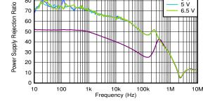
$V_{IN}$  = 1.4 V,  $I_{OUT}$  = 1 A,  $C_{OUT}$  = 47  $\mu F$  || 10  $\mu F$  || 10  $\mu F,$ C<sub>NR/SS</sub> = 10 nF, C<sub>FF</sub> = 10 nF
