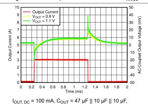
Figure 6-17. Load Transient vs Time and V<sub>OUT</sub> Without Bias
