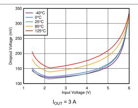
Figure 6-20. Dropout Voltage vs V<sub>IN</sub> Without Bias
