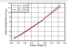
$V_{IN} = V_{OUT} + 0.3 \text{ V}$  and  $V_{BIAS} = 5 \text{ V}$  for  $V_{OUT} \le 2.2 \text{ V}$ ,  $C_{OUT} = 47 \ \mu\text{F} \parallel 10 \ \mu\text{F} \parallel 10 \ \mu\text{F}$ ,  $C_{NR/SS} = 10 \ n\text{F}$ ,  $C_{FF} = 10 \ n\text{F}$ , RMS noise BW = 10 Hz to 100 kHz
