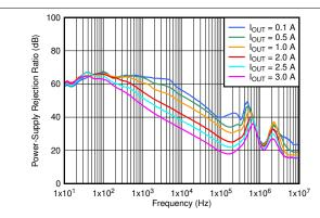
$V_{IN}$  = 1.1 V,  $V_{BIAS}$  = 5 V,  $C_{OUT}$  = 47  $\mu F$  || 10  $\mu F$  || 10  $\mu F$  ,  $C_{NR/SS}$  = 10 nF,  $C_{FF}$  = 10 nF
