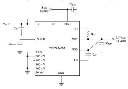
Figure 8-2. ANY-OUT Configuration Circuit (TPS7A8400A) (3.3-V Output, No External Bias)
