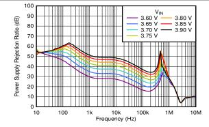
$I_{OUT}$  = 3 A,  $C_{OUT}$  = 47  $\mu$ F || 10  $\mu$ F || 10  $\mu$ F,  $C_{NR/SS}$  = 10 nF, C<sub>FF</sub> = 10 nF
