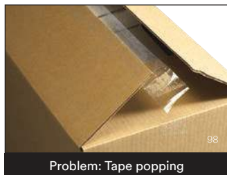
Problem: Tape popping
