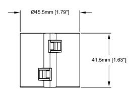
TO DISENGAGE: PLACE FLAT HEAD SCREWDRIVER HERE AND TURN COUNTER-CLOCKWISE.
