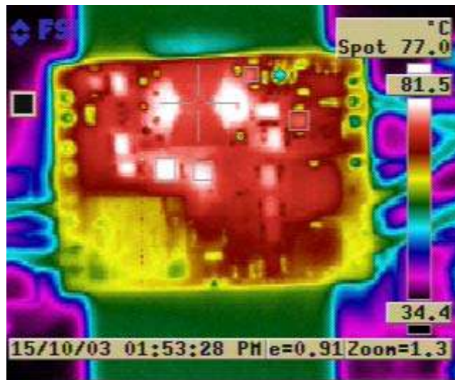
FIGURE 15. THERMAL IMAGE: 48V INPUT, 300LFM AIR FLOW
