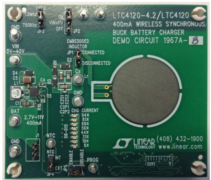
Figure 14. Rx Layout with Ferrite Shield: Demo Circuit 1967A-B
