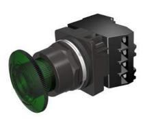
30mm BlackMax, Epoxy Coated Corrosion Resistant Complete Metal Unit Illuminated Twist-to-Release Full Voltage, 120V AC/DC Incandescent Lamp Mushroom Head Cap Small 1.79" (45 mm) Plastic Cap, Green 2 Position Maintained, Twist-to-Release with 1 N.O. - 1 N.C. Heavy Duty Contacts, A600/P600 UL Listed, CSA Certified NEMA 1,3,3R,4,4X,12,13 & Automotive Standards
