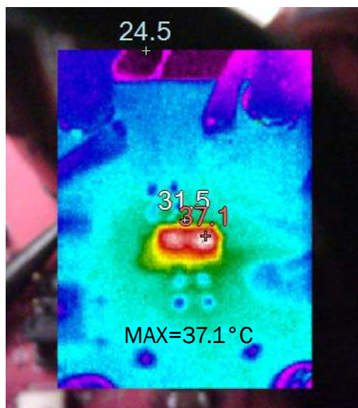
FIGURE 21. THERMAL IMAGE AT V_{IN} = 5V , V_{OUT} = 1.2V , I_{OUT} = 3A , f_{SW} = 1.5MHz , T_A = +25^\circ C , FREE AIR 0 LFM
