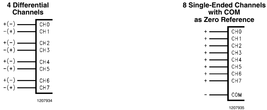
FIGURE 9. Input Multiplexer Options
