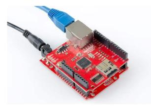
An Ethernet Shield piggybacks onto a RedBoard to help get it connected to the Internet.
