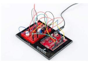
A tangled assortment of jumper wires run between the RedBoard headers and components on a breadboard. An Arduino baseplate holds them all in one place.
