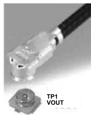
Figure 8. Technique for Measuring Output Ripple and Step Response with a Low Inductance Connector (Not Supplied)
