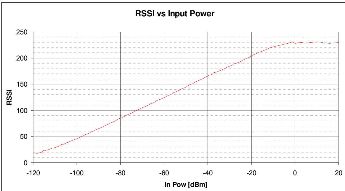
Figure 30. RSSI Value vs. Input Power
