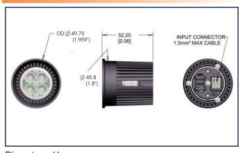
Diameter x H 49.75mm x 52.25mm (1.959" x 2.06") Maximum Cable Dia - 1.5mm<sup>2</sup> / 16 AWG
