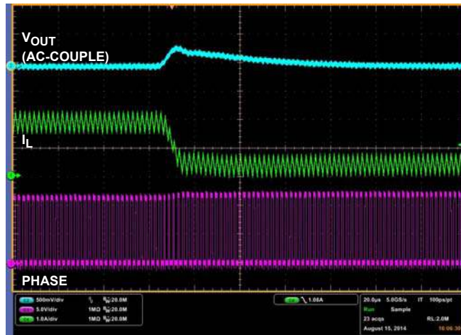
FIGURE 12. LOAD TRANSIENT RESPONSE
