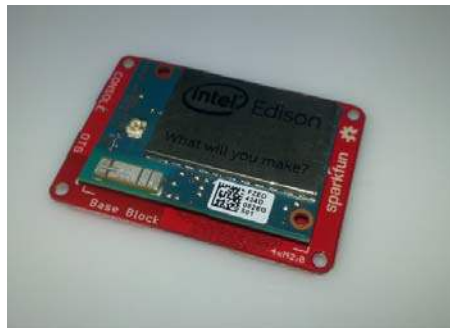
Base Block Installed
