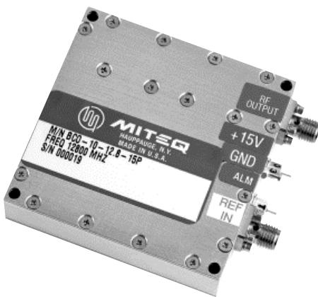
The BCO Series phase-locked source offers excellent phase noise and spurious performance in a 2.25"W x 2.25"L x .6"H housing. Available in fixed frequencies from 200 MHz to 16 GHz in fundamental or multiplied configurations. Units can operate from either external reference, or internal TCXO with stability up to 1 ppm. Available with operating voltages from 5.2 to 15 VDC, and feedthru filtercons or a 4 pin interface connector.
