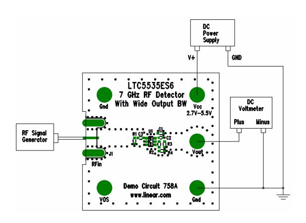
Figure 1. Proper Measurement Equipment Setup
