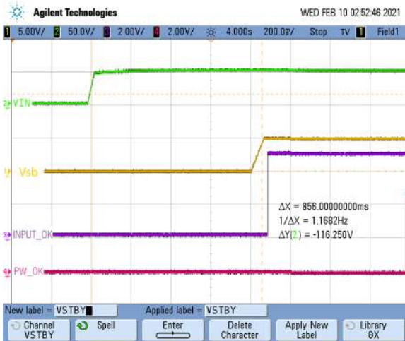
Figure 7: Turn-on Delay; Vin to Vsb delay; back
