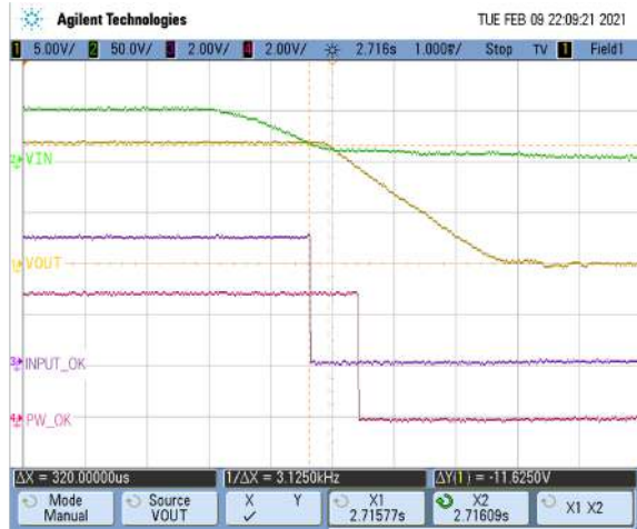
Figure 5: Turn off by Vin removal; Input_OK to Vout Delay; Back
