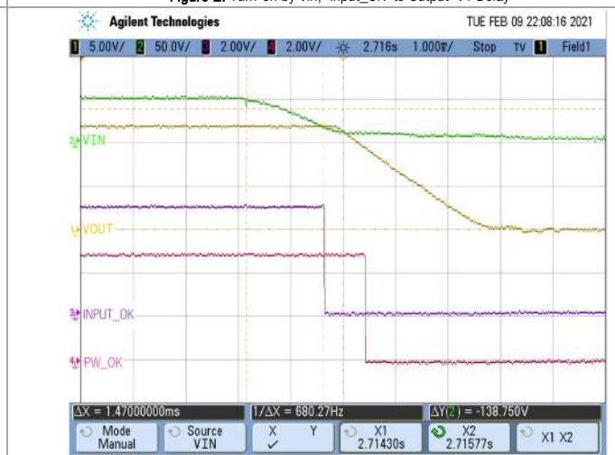
Figure 4: Turn-off by Vin removal; Input to Input_OK delay; Back
