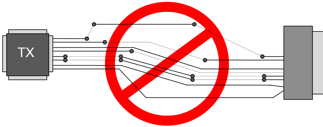
Figure 19. Example of Incorrect Differential Signal Routing
