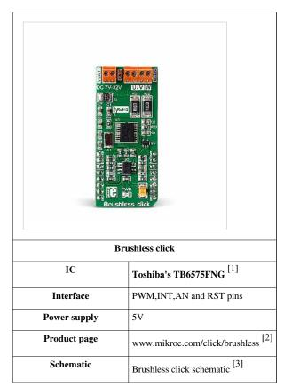
Brushless click carries Toshiba's TB6575FNG IC for driving 3-phase full-wave Brushless DC motors — which are ideal for powering flying drones. The click is able to safely drive external motors with up to 32V/2A.
