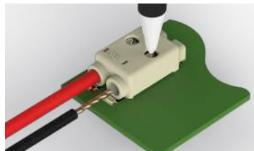
Insert stranded conductors horizontal to printed circuit boards and/or remove both solid and stranded conductors by first depressing the release mechanism with a ball point pen or the tip of any small device. Remove the conductors by pulling horizontal to the printed circuit board.
