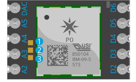
When two radios occupying the same frequency band are used in the same system, such as Wi-Fi and Bluetooth, a coexistence interface can be used to coordinate transmit activity, to ensure optimal performance by arbitrating conflicts between the two radios.
