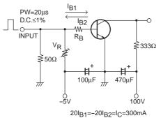
20I<sub>B1</sub>=-20I<sub>B2</sub>=I<sub>C</sub>=300mA (For PNP, the polarity is reversed.)
