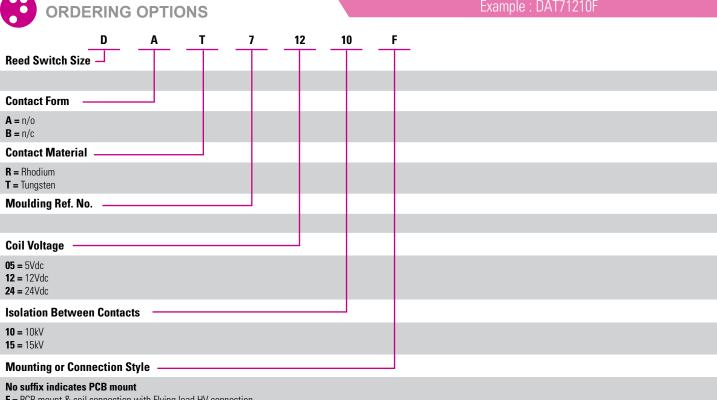
**F** = PCB mount & coil connection with Flying lead HV connection
