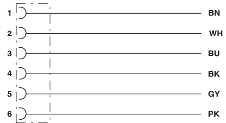
Contact assignment of M8 socket
