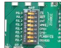
Figure 6-3: Switch 8 on the DIP switch SW15 is in ON position, DS1820 is connected to the P2.7 pin
