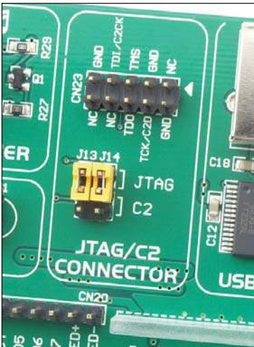
Figure 3-3: Connector for programmer
