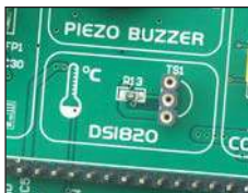
Figure 6-1: DS1820 connector (DS1820 is not connected)
