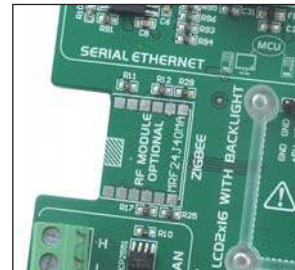
Figure 10-2: Connector for ZigBee module
