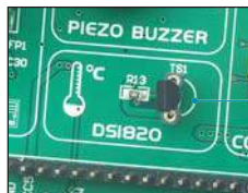
Figure 6-2: Temperature sensor DS1820 is connected
