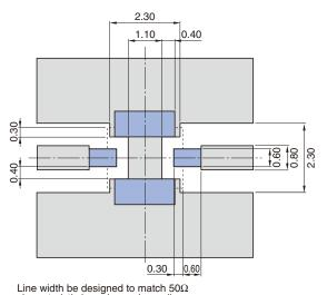
Line width be designed to match  $50\Omega$  characteristic impedance depending on PCB material and thickness.
