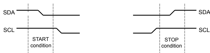
Figure 16-3. START and STOP Conditions
