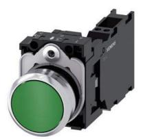
Pushbutton, 22 mm, round, metal, shiny, green, pushbutton, flat, momentary contact type, 1 NO+1 NC, Spring-type terminal
