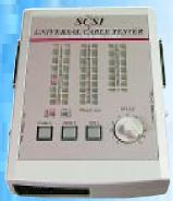
This SCSI tester can test cable with up to 68 lines. With the optional PC or MAC cable Test Unit it can be upgraded to a multi cable tester. The transmitted and received data between the two ends of the cable will be compared. The result is shown by LEDs.
