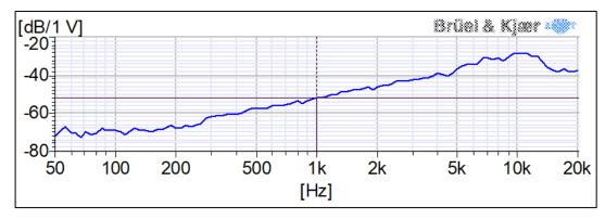
Typical Frequency Response Near-Field vs. Far-Field (2.54cm vs 50cm)
