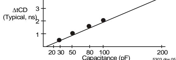
Figure 2. Lumped Capacitive Load, Typical Derating
