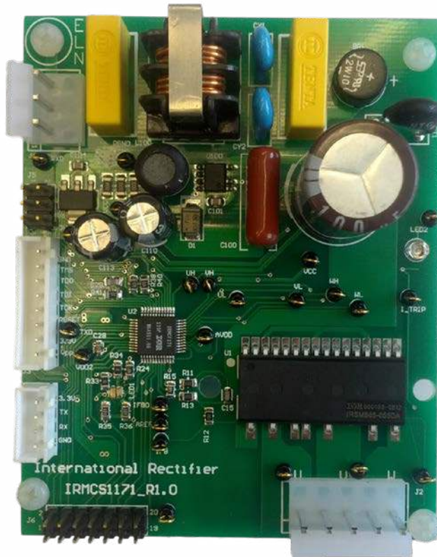
Figure 4: Reference design board featuring the \mu IPM™-DIP module and the iMotion™ IRMC5171 digital control IC
