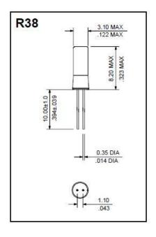
NOTE: Through hole device can withstand 245°C soldering by terminals only
