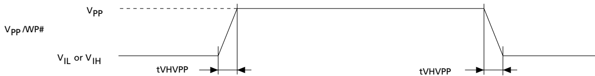
Figure 24: Accelerated Programming Timing Waveform
