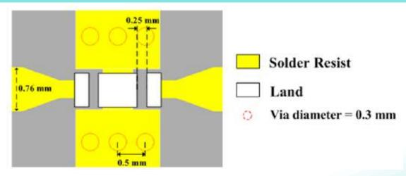
Line width should be designed to match  $50\Omega$  characteristic impedance, depending on PCB material and thickness.
