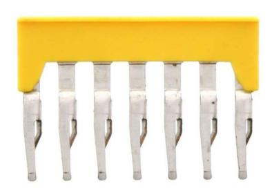
Insulated cross-connector, No. of poles: 7, Mounting type: Plug in, Width: 34.6 mm, Rated cross-section: 2.5 mm², Colour: Yellow
