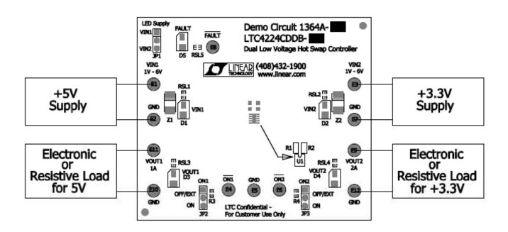
Figure 1. Proper Measurement Equipment Setup
